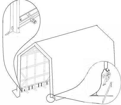
Hang the endwall with bungee ball the the frame door .,Use 6x180mm to fix the skirt to ground .
