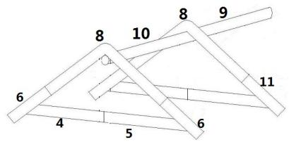
D. Insert corner arch No.7 to extension bar No. 6 and No.11 .Do to keep at least one person to keep the structure in upright direction . Use Screw 2.5" to connect No.6 to 7.
