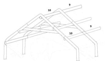
F. Insert leg No.1 and No.2 in to the corner arch .And connect them by cross bar no.10 and no.9 with screws (4" screw ). No. 9 is for add-on sections . Also at this point, use diagonal 3 to make the frame stable. Any position to put on diagonal 3, use screw 4.5".
